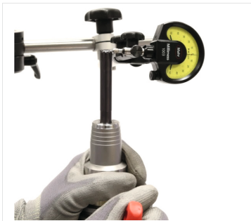
Fig. 17: Adjusting the radial run-out
