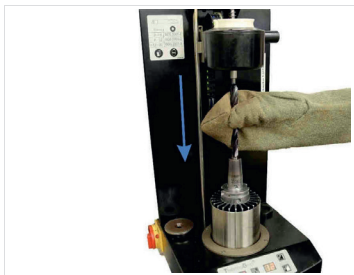
Fig. 8: Insert tool into the location bore
