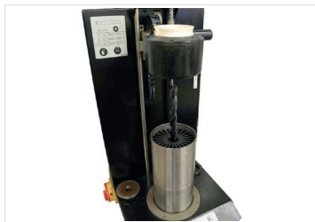
Fig. 9: Cool the shrink chuck with tool
