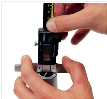
Fig. 6: Set shrink chuck to tool length
