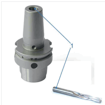
Fig. 5: Clean the shrink chuck and tool
