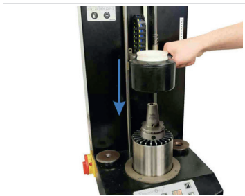
Fig. 7: Heat the shrink chuck with shrink unit
