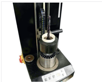
Fig. 10: Heat the shrink chuck with tool
